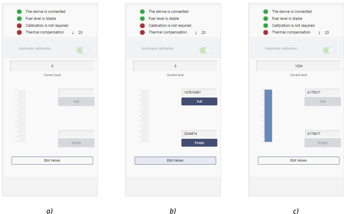
Fig. 19 – Empty/full FLS calibration section.
